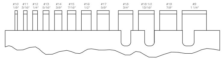
The cutouts in the blade holder adjacent to the #18, #18 1/2 and #9 blades are to accommodate the depth stops on the match and sash blades in the second layer.
