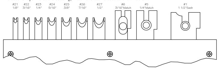
When assembling the box, ensure that the narrow slots in each layer are aligned with each other so that the match and sash blades will align with the cutouts in the first layer.
